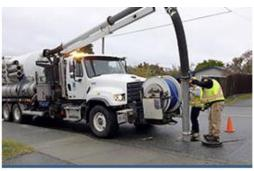
Sewer main cleaning is also done for CCTV inspection work. These inspections allow us to see the condition of our sewer mains and make necessary repairs or replacements.
